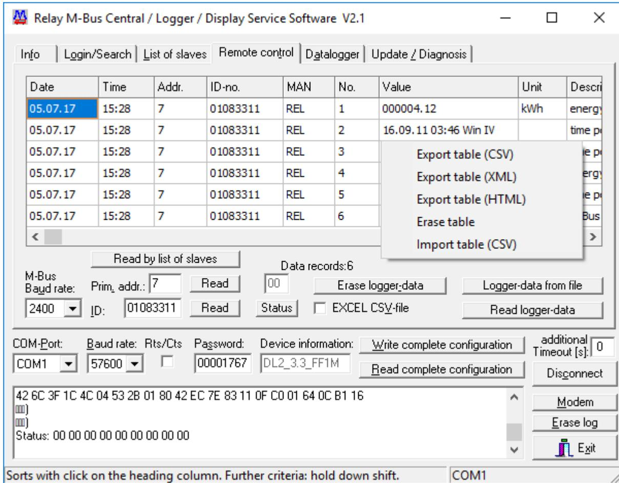
The "Remote control"-sheet is the central sheet for remote reading of M-Bus meters with known addresses and for downloading logger-data from the master models MR004DL, MR005DL, MR006DL, DR001 and DR002. Meter data is transferred to the table containing timepoint of reading, address, medium, measured value and other information.
