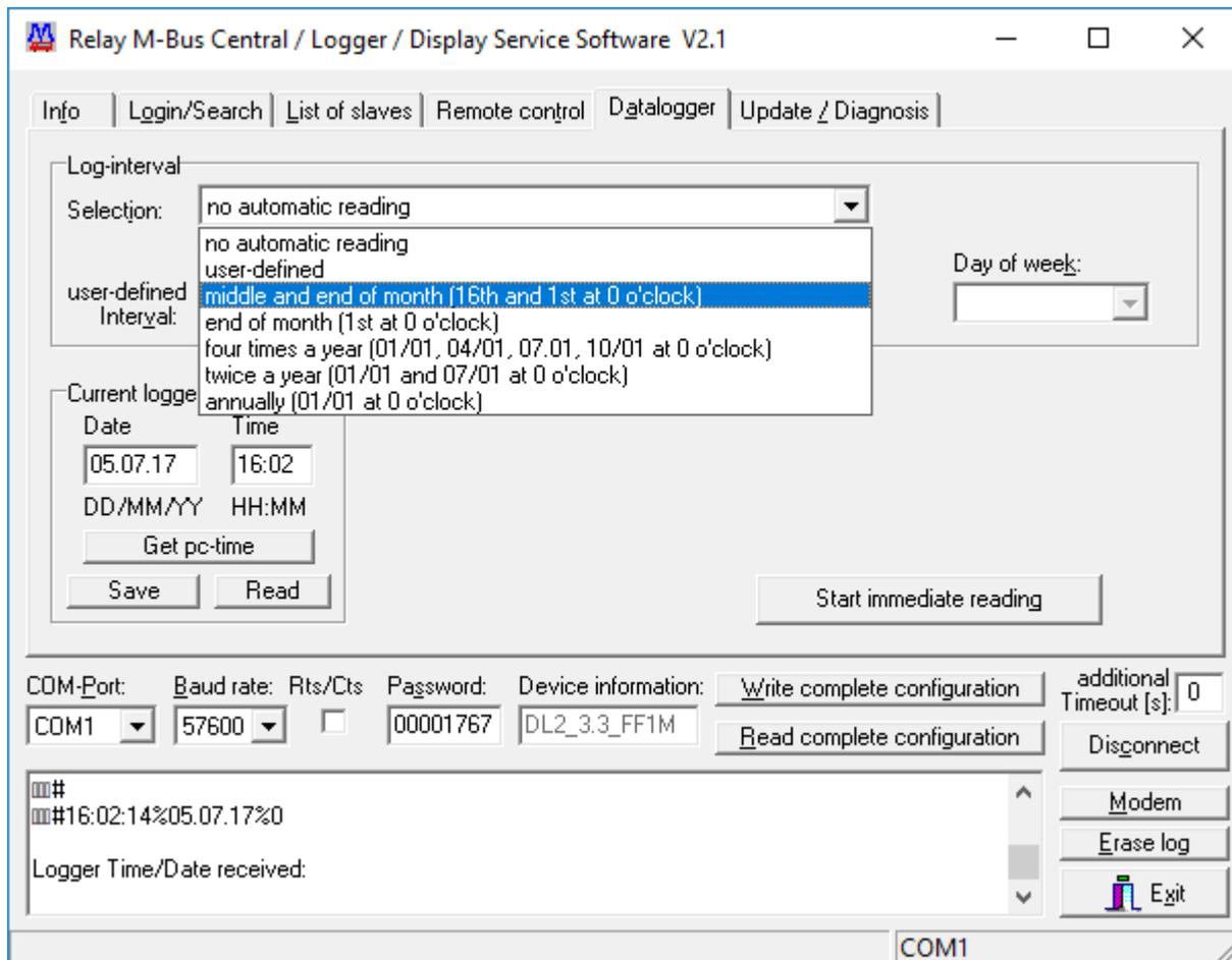
The "Datalogger"-sheet contains the settings for the log-strategy. The group-field "Log-interval" provides a setup of the M-Bus read-out time. Predefined or user-defined time intervals from a few minutes to a whole year are possible.
