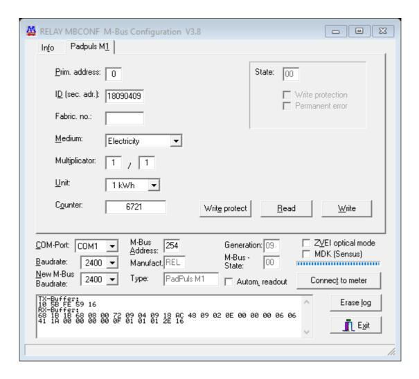
This sheet shows the current settings and values of the PadPuls M1. The following input boxes and buttons are used to change the parameters of the pulse adapter:
