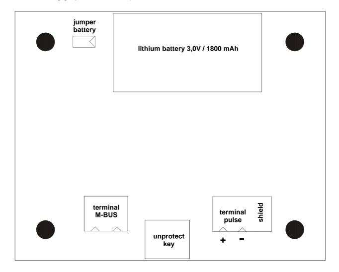
**Attention:** The battery jumper is plugged in at the factory and should not be removed as the PadPuls M1 will otherwise lose configuration. In this case, a new configuration including programming of the ID is necessary.
