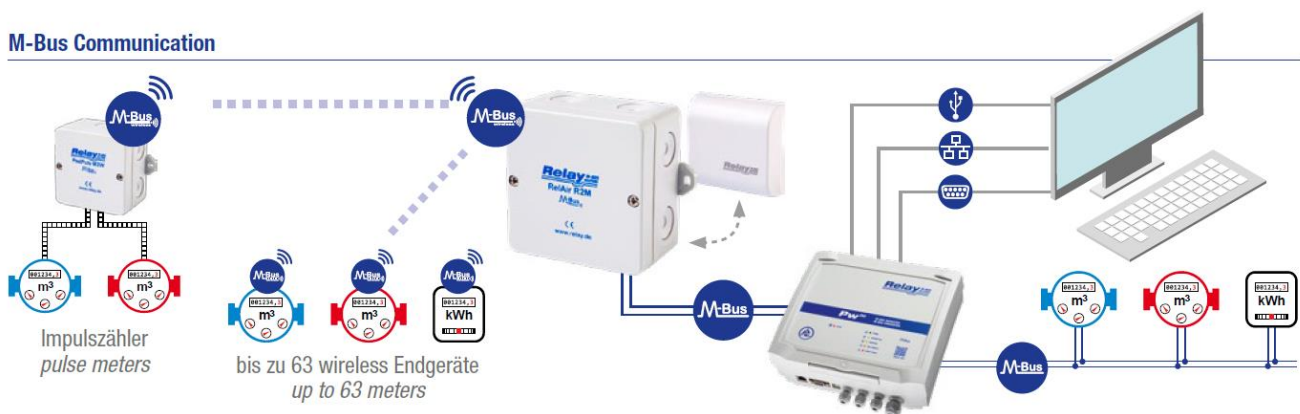
Picture: Wireless M-Bus system with PadPuls M2W, RelAir R2M Gateway and PW250
